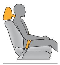
Adjusting a head restraint so the center is level with the back of the occupant's head (or as high as possible for taller people) can help reduce injuries during a rear impact.
