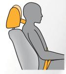
In vehicles equipped with active head restraints, the restraint will move up and forward a little when enough pressure is applied against the seat-back.
