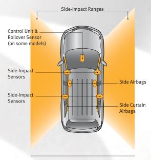
On average, side impacts account for about onefourth of all crash fatalities. Side Airbags: During a side impact, sensors detect the crash and send information to the control unit. If the impact is severe enough, the control unit signals the driver's or the front passenger's side airbag to instantly inflate into the space between the door and the occupant.
