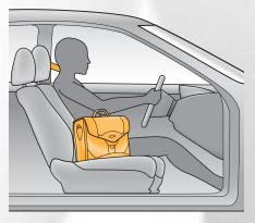
If sensors detect up to about 67 lbs (the weight of an infant or small child) on the front passenger's seat, the airbag will automatically turn off.
