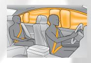
Side curtain airbags can help protect the heads of outboard occupants during a side impact.
